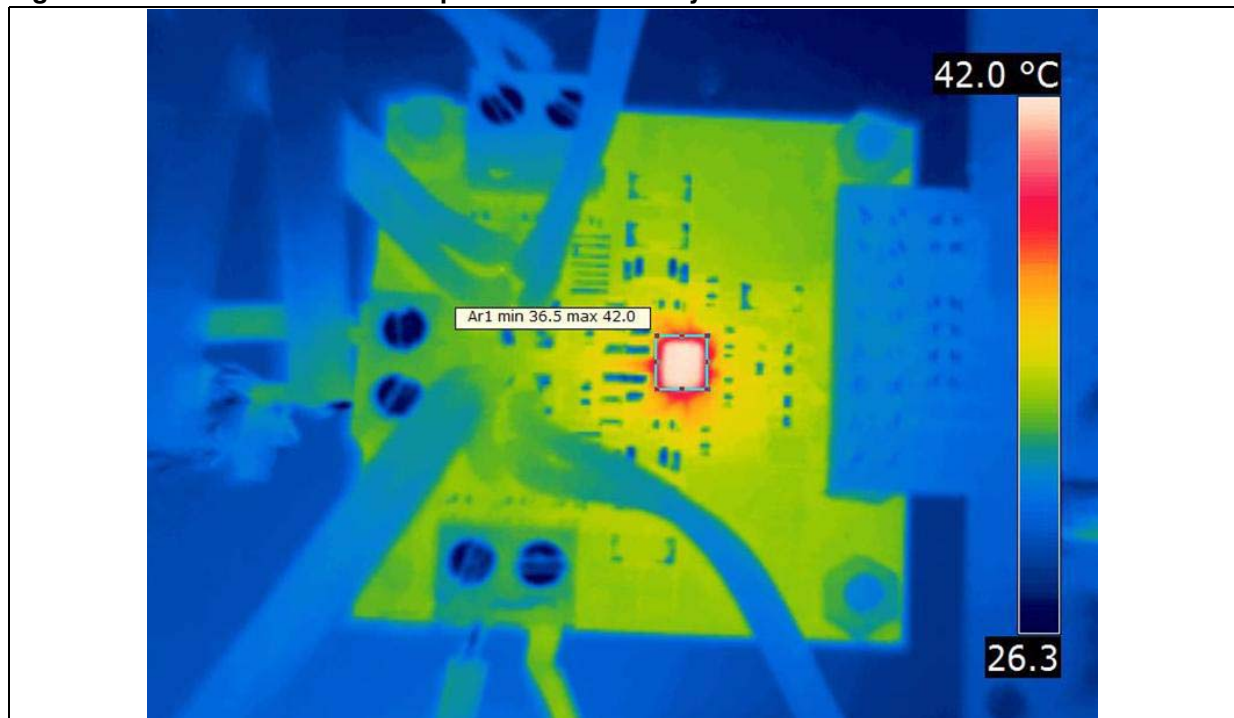
Figure 4. STA333IS: 500 mA output current and 4-layer PCB - thermal measurement
