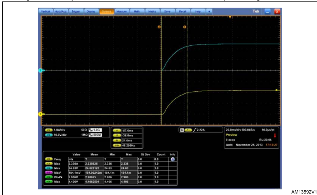
Figure 34. Output short circuit (hiccup mode)
