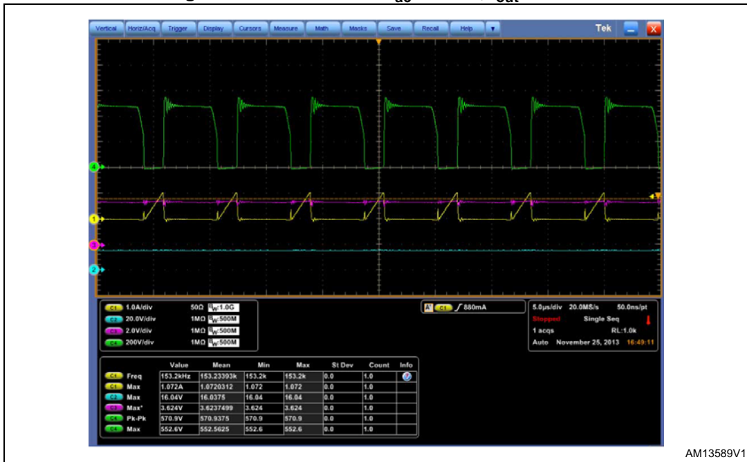
Figure 30. Condition 15: V_{ac} = 265\text{ V} ; I_{out} = 1.8\text{ A}
