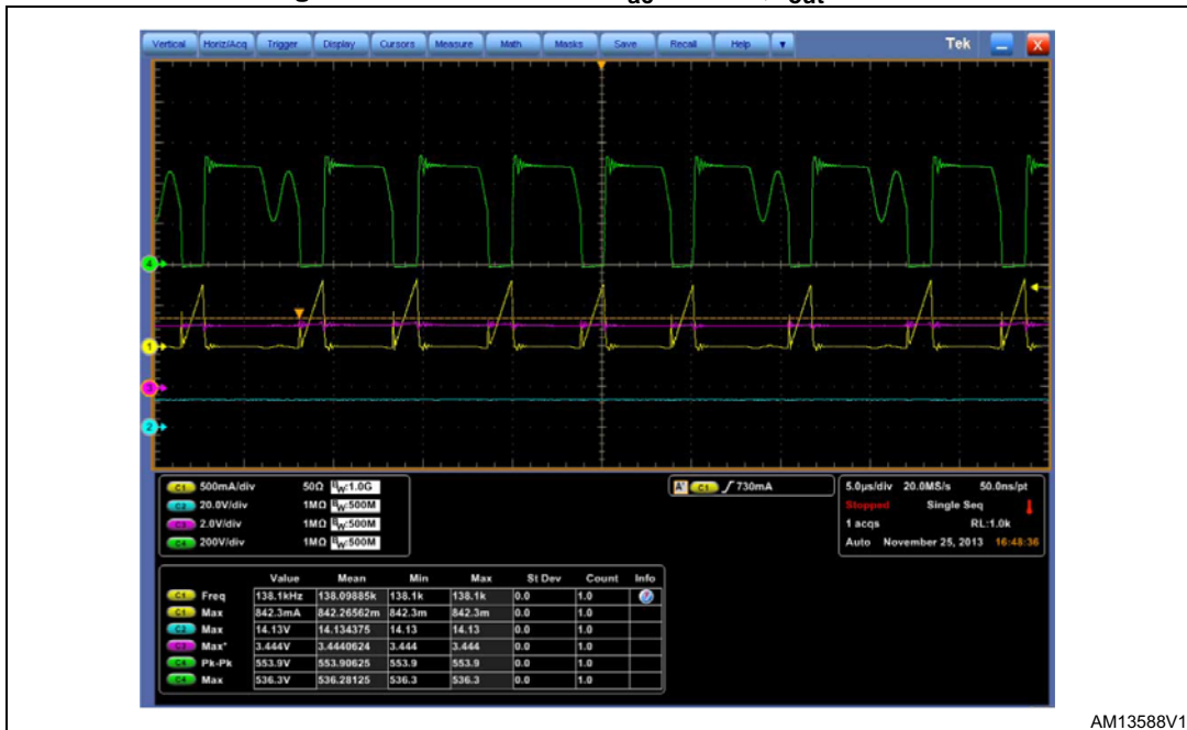
Figure 30. Condition 15: V_{ac} = 265\text{ V} ; I_{out} = 1.8\text{ A}
