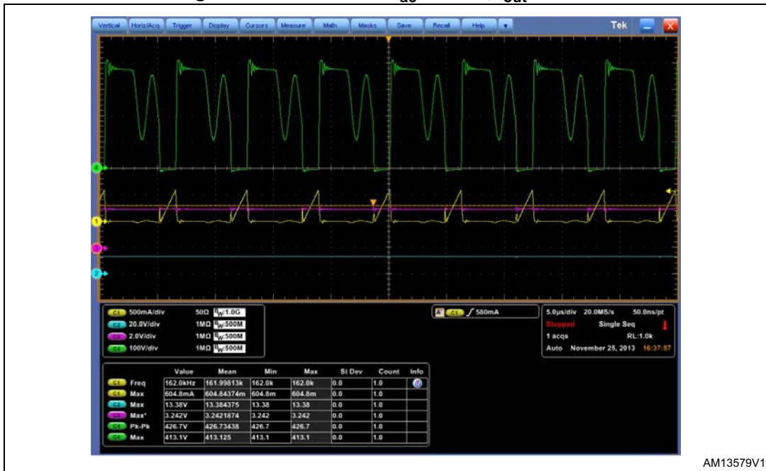
Figure 20. Condition 5: V_{ac} = 180\text{ V} ; I_{out} = 0.6\text{ A}
