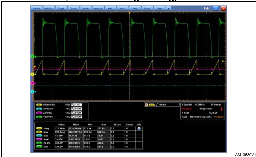
Figure 22. Condition 7: V_{ac} = 180\text{ V} ; I_{out} = 1.8\text{ A}
