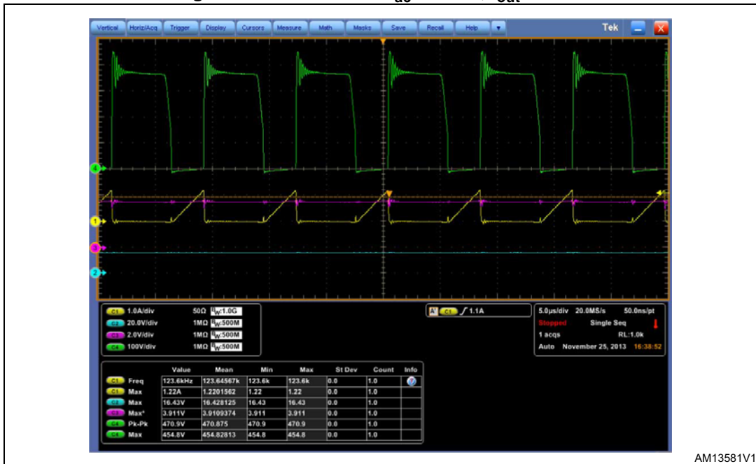
Figure 22. Condition 7: V_{ac} = 180\text{ V} ; I_{out} = 1.8\text{ A}
