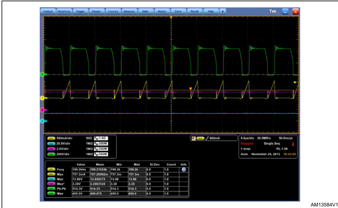
Figure 26. Condition 11: V_{ac} = 230\text{ V} ; I_{out} = 1.8\text{ A}
