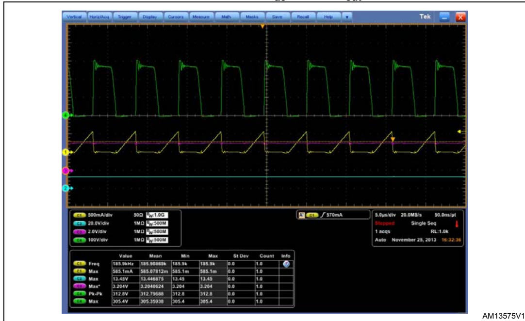
Figure 16. Condition 1: V ac = 100 V; I out = 0.6 A
