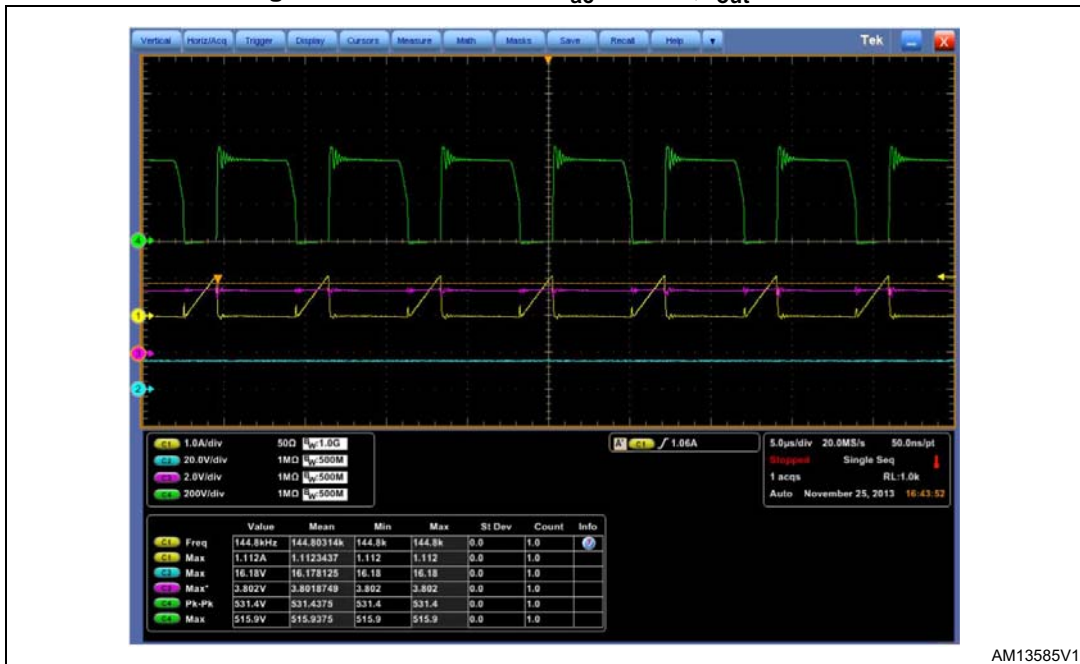
Figure 26. Condition 11: V_{ac} = 230\text{ V} ; I_{out} = 1.8\text{ A}
