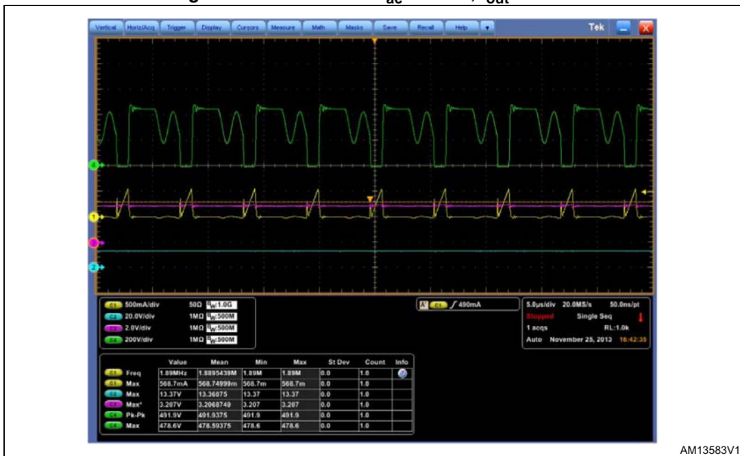
Figure 24. Condition 9: V_{ac} = 230\text{ V} ; I_{out} = 0.6\text{ A}
