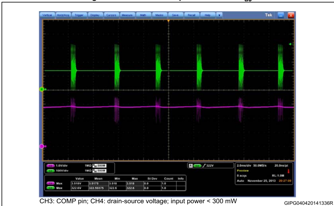
Figure 38. Burst mode operation at 100 V ac
