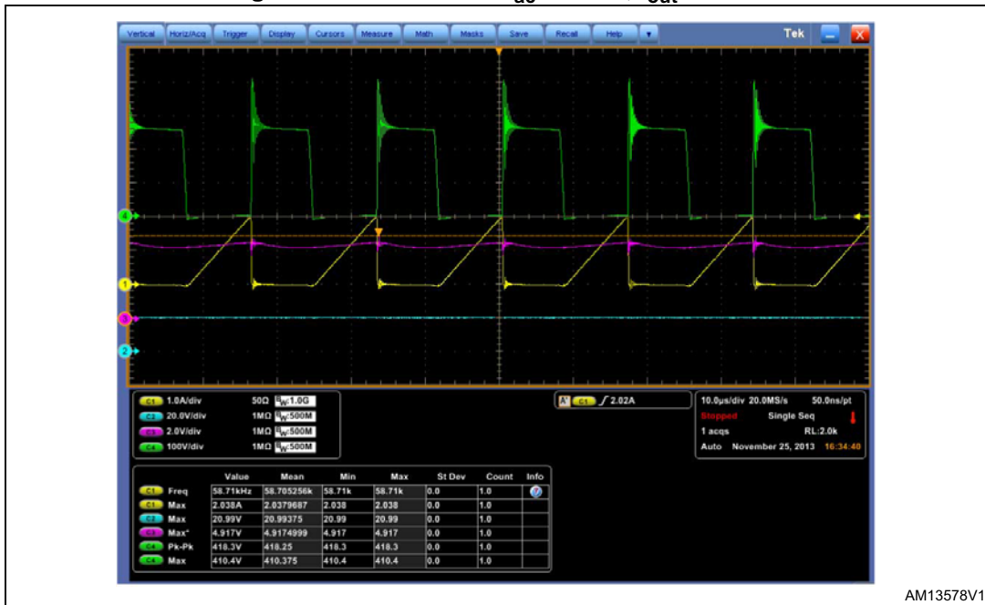
Figure 20. Condition 5: V_{ac} = 180\text{ V} ; I_{out} = 0.6\text{ A}
