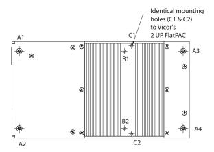
Maximum allowable torque is 5 in. lbs.,. The maximum penetration for mounting holes A1, A2, A3 and A4 is 0.125 in. (3mm) and for mounting holes B1, B2, C1 and C2 is 0.250 in. (6mm). The minimum recommended mounting holes are as follows:
