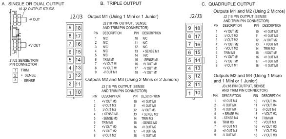
**Figure 3: Output Power Connections**
