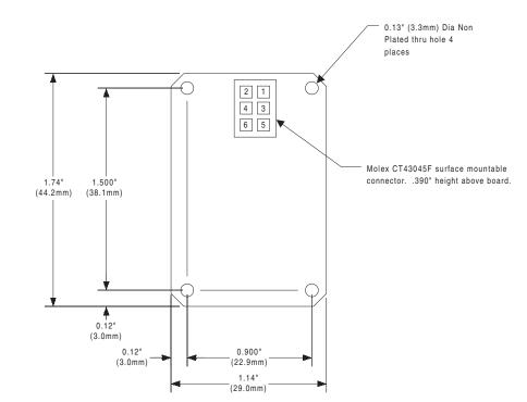
Figure 2. Mechanical Drawing
