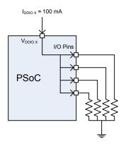
Conversely, for the 100-pin and 68-pin devices, the set of I/O pins associated with any VDDIO may sink up to 100 mA total, as shown in Figure 2-2.
