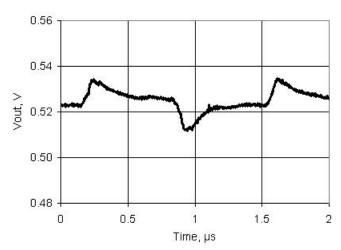
Figure 11-55. VDAC Voltage Noise, 1 V Mode, High speed mode,  $V_{\rm DDA}$  = 5 V
