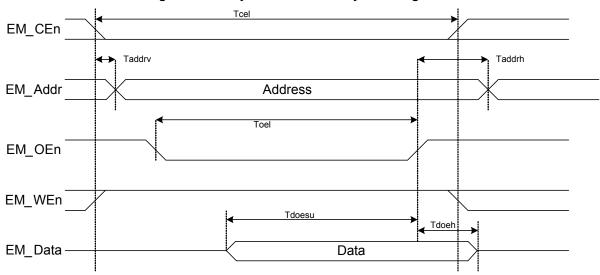
Table 11-61. Asynchronous Read Cycle Specifications
