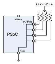
For the 48-pin devices, the set of I/O pins associated with VDDIO0 plus VDDIO2 may sink up to 100 mA total. The set of I/O pins associated with VDDIO1 plus VDDIO3 may sink up to a total of 100 mA.
