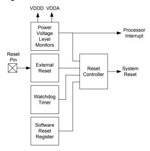
The term **device reset** indicates that the processor as well as analog and digital peripherals and registers are reset.
