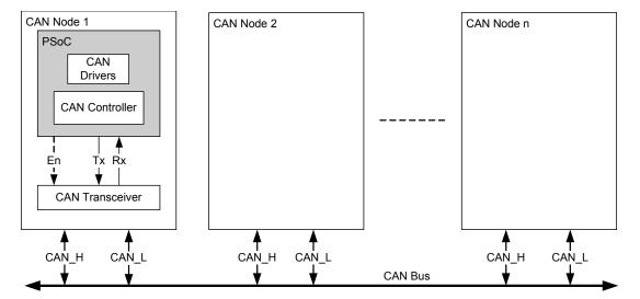
Figure 7-14. CAN Bus System Implementation
