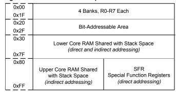
In addition to the register or bit address modes used with the lower 48 bytes, the lower 128 bytes can be accessed with direct or indirect addressing. With direct addressing mode, the upper 128 bytes map to the SFRs. With indirect addressing mode, the upper 128 bytes map to RAM. Stack operations use indirect addressing; the 8051 stack space is 256 bytes. See the "Addressing Modes" section on page 12
