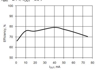
Figure 11-10. Efficiency vs  $V_{OUT}$  I<sub>OUT</sub> = 30 mA,  $V_{BAT}$  = 0.6 V and 1.2 V
