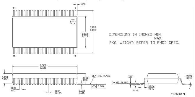
Figure 13-1. 48-pin (300 mil) SSOP Package Outline
