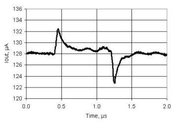
Figure 11-43. IDAC Current Noise, 255  $\mu$ A Mode, Source Mode, High speed mode, V<sub>DDA</sub> = 5 V
