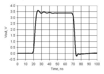
Figure 11-17. SIO Output Rise and Fall Times, Slow Strong Mode,  $V_{\rm DDIO}$  = 3.3 V, 25 pF Load
