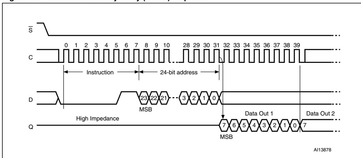
If Chip Select ( $\overline{S}$ ) continues to be driven low, the internal address register is incremented automatically, and the byte of data at the new address is shifted out.
