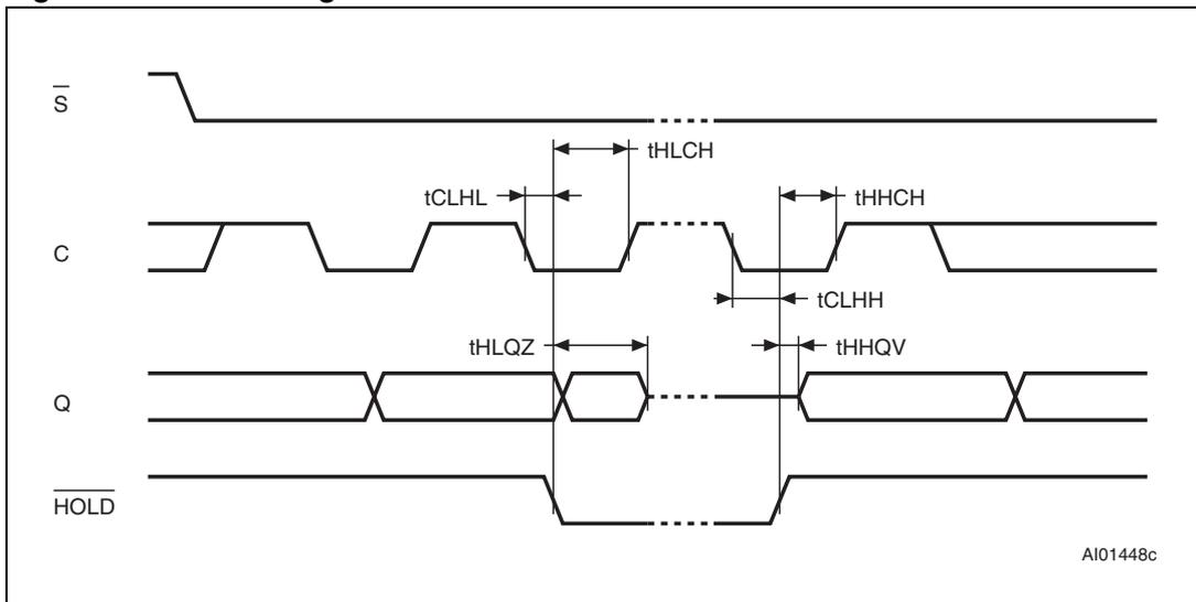
Figure 22. Serial output timing
