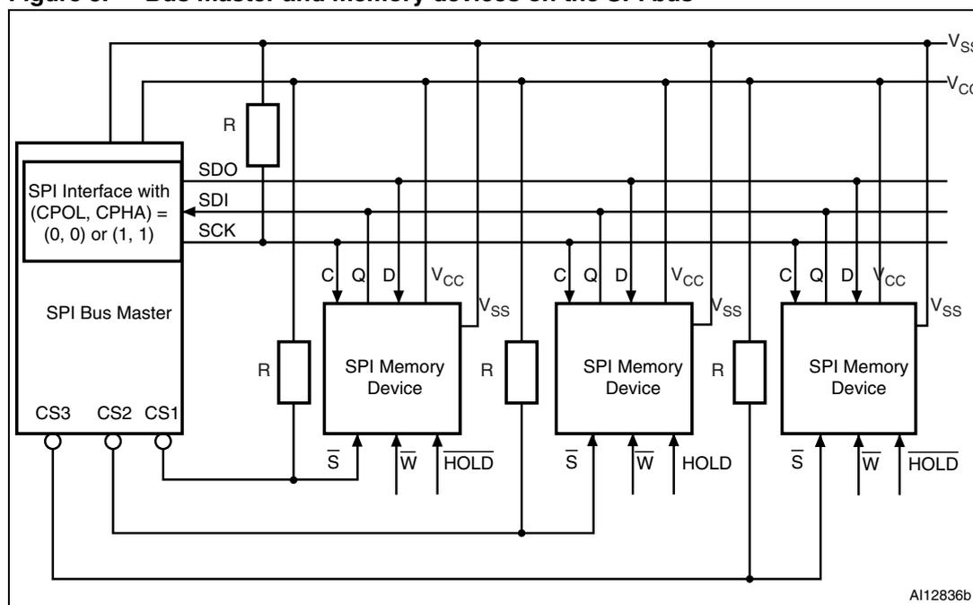
1. The Write Protect ( $\bar{W}$ ) and Hold ( $\overline{\text{HOLD}}$ ) signals should be driven, high or low as appropriate.
