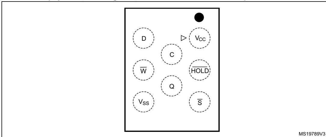
**Caution:** As EEPROM cells lose their charge (and so their binary value) when exposed to ultra violet (UV) light, EEPROM dice delivered in wafer form or in WLCSP package by STMicroelectronics must never be exposed to UV light.
