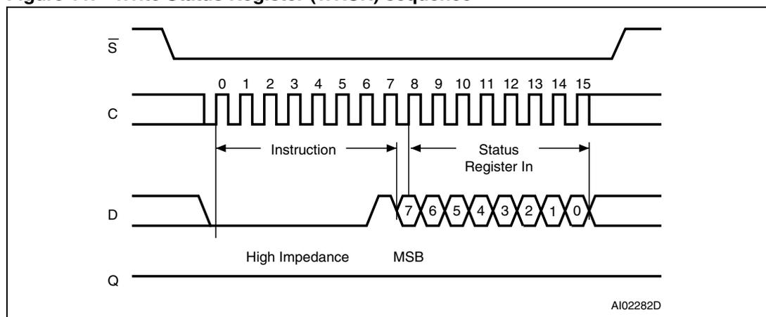
Driving the Chip Select ( $\overline{S}$ ) signal high at a byte boundary of the input data triggers the self-timed Write cycle that takes  $t_{WV}$  to complete (as specified in AC tables under [Section 9: DC and AC parameters](#)).
