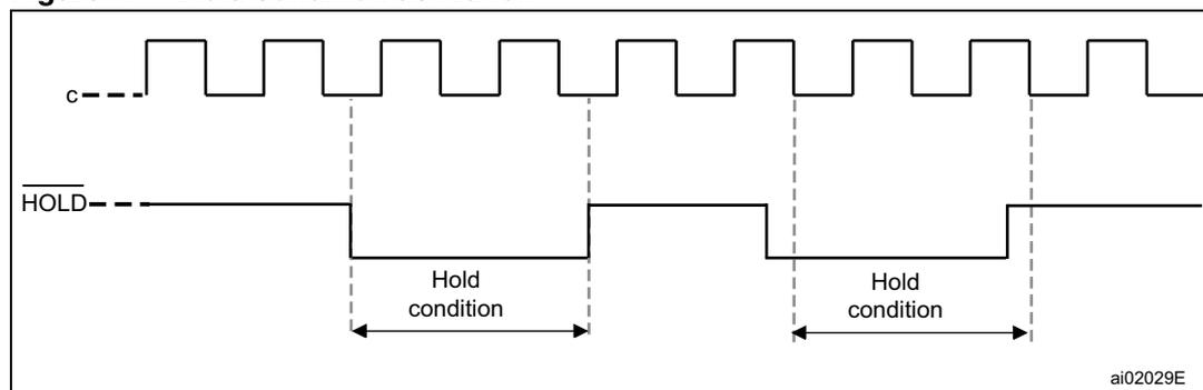
The Hold condition starts when the Hold ( $\overline{HOLD}$ ) signal is driven low when Serial Clock (C) is already low (as shown in [Figure 7](#)).
