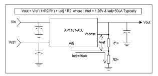
The AP1187 keeps a constant 1.25V between the VSENSE pin and the ADJ pin. By placing a resistor R1 across these two pins and connecting the VSENSE and VOUT pin together, a constant current flows through R1, adding to the IADJ current and into the R2 resistor producing a voltage equal to the (1.25/R1)\*R2 + IADJ\*R2. This voltage is then added to the 1.25V to set the output voltage. This is summarized in the above equation.
