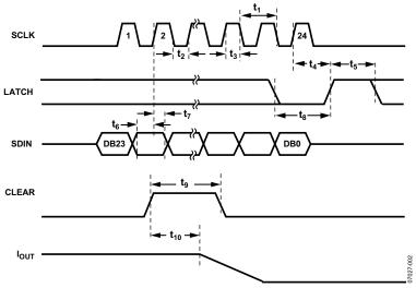
Figure 2. Write Mode Timing Diagram
