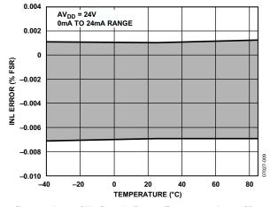
Figure 10. Integral Nonlinearity Error vs. Temperature, Internal RSET
