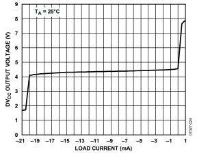
Figure 27. DV<sub>CC</sub> Output Voltage vs. Load Current
