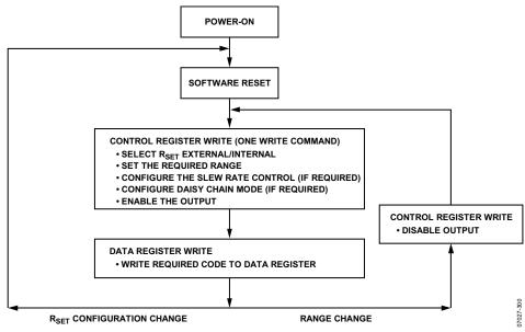
Figure 40. Programming Sequence to Write/Enable the Output Correctly
