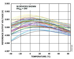
Figure 32. Reference Output Voltage vs. Temperature
