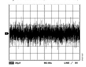
Figure 30. Reference Noise (100 kHz Bandwidth)
