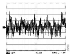
Figure 29. Reference Noise (0.1 Hz to 10 Hz Bandwidth)
