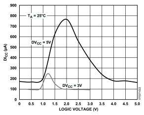
Figure 25. DIcc vs. Logic Input Voltage
