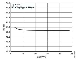
Figure 50. R3 Resistor Value vs. IOUT
