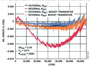
Figure 7. Integral Nonlinearity Error vs. Code
