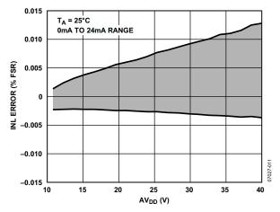
Figure 16. Integral Nonlinearity Error vs. AV<sub>DD</sub>, External R<sub>SET</sub>
