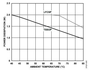
Figure 53. Maximum Power Dissipation vs. Ambient Temperature
