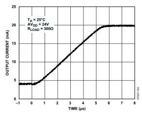
Figure 36. 4 mA to 20 mA Output Current Step
