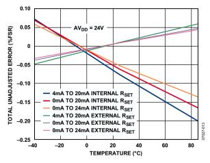
Figure 13. Total Unadjusted Error vs. Temperature
