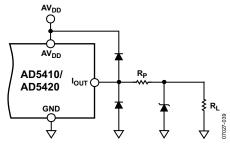
Figure 51. Output Transient Voltage Protection
