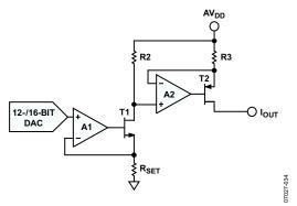
Figure 38. Voltage-to-Current Conversion Circuitry
