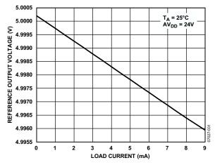
Figure 34. Reference Output Voltage vs. Load Current
