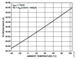
Figure 49. R3 Resistor Value vs. Temperature
