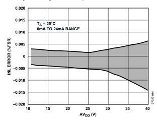
Figure 17. Integral Nonlinearity Error vs. AV<sub>DD</sub>, Internal R<sub>SET</sub>
