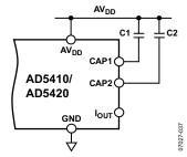
Figure 44. IOUT Filtering Capacitors
