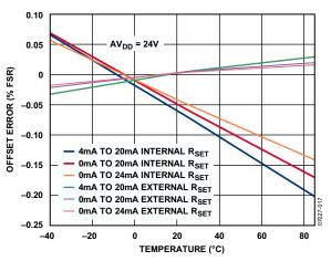
Figure 14. Offset Error vs. Temperature
