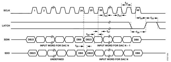
Figure 4. Daisy-Chain Mode Timing Diagram
