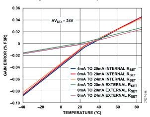
Figure 15. Gain Error vs. Temperature
