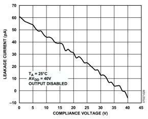
Figure 31. Output Leakage Current vs. Compliance Voltage
