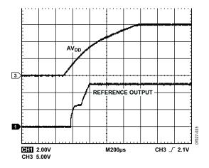
Figure 28. Reference Turn-on Transient
