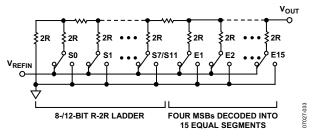
Figure 37. DAC Ladder Structure
