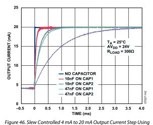
External Capacitors on the CAP1 and CAP2 Pins
