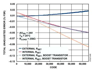
Figure 9. Total Unadjusted Error vs. Code
