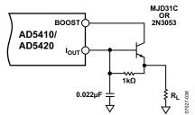
Figure 41. External Boost Configuration
