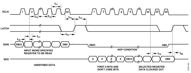
Figure 3. Readback Mode Timing Diagram
