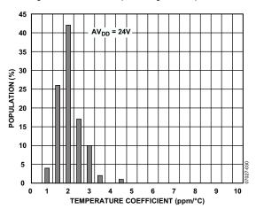
Figure 33. Reference Temperature Coefficient Histogram
