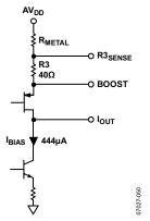
Figure 48. Structure of Current Output Circuit
