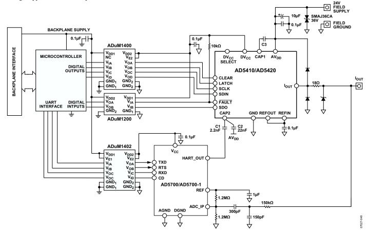
Figure 55. AD5410/AD5420 in an Industrial Analog Output Application
