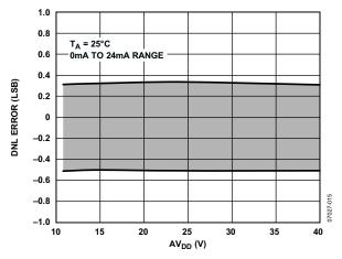
Figure 19. Differential Nonlinearity Error vs.  $AV_{DD}$ , Internal  $R_{SET}$
