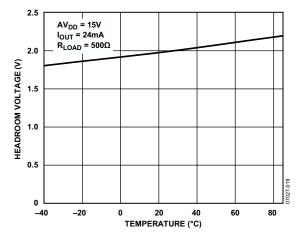
Figure 22. Compliance Voltage Headroom vs. Temperature
