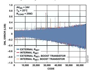
Figure 8. Differential Nonlinearity Error vs. Code
