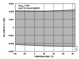
Figure 11. Integral Nonlinearity Error vs. Temperature, External R<sub>SET</sub>
