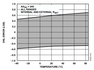
Figure 12. Differential Nonlinearity Error vs. Temperature
