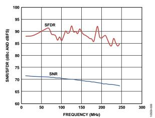
Figure 9. AD9250-170 Single-Tone SNR/SFDR vs. Input Frequency (f<sub>IN</sub>)
