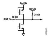
Figure 35. Equivalent RST Input Circuit
