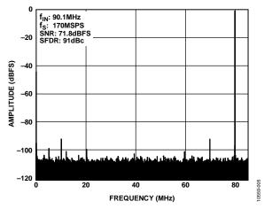
Figure 5. AD9250-170 Single-Tone FFT with  $f_{IN} = 90.1$  MHz
