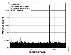
Figure 23. AD9250-250 Two-Tone FFT with  $f_{\rm IN1}=89.12$  MHz,  $f_{\rm IN2}=92.12$  MHz,  $f_{\rm S}=250$  MSPS
