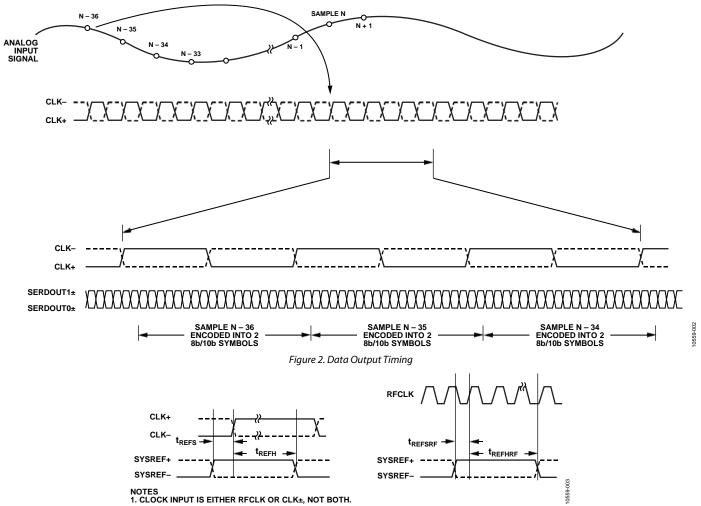
Figure 3. SYSREF± Setup and Hold Timing
