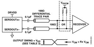
Figure 57. AC-Coupled Digital Output Termination Example
