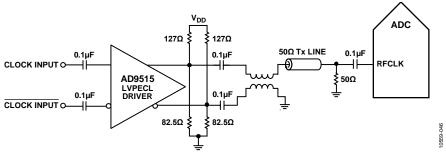
Figure 50. Differential PECL RF Clock Input Circuit
