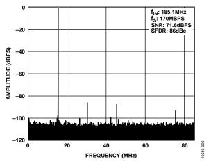
Figure 6. AD9250-170 Single-Tone FFT with  $f_{IN} = 185.1$  MHz
