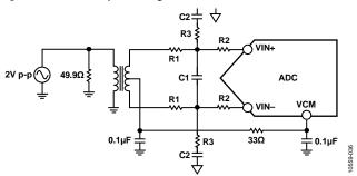
Figure 40. Differential Transformer-Coupled Configuration
