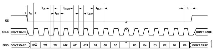
Figure 62. Serial Port Interface Timing Diagram
