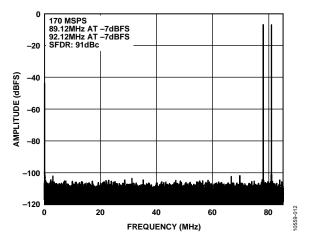
Figure 12. AD9250-170 Two-Tone FFT with  $f_{\rm IN1}$  = 89.12 MHz,  $f_{\rm IN2}$  = 92.12 MHz,  $f_{\rm S}$  = 170 MSPS
