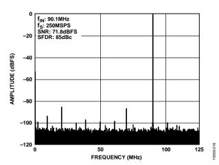
Figure 16. AD9250-250 Single-Tone FFT with  $f_{\text{IN}}$  = 90.1 MHz
