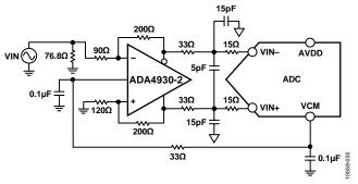
Figure 39. Differential Input Configuration Using the ADA4930-2
