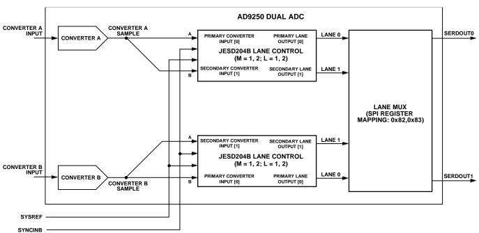
Figure 54. AD9250 Transmit Link Simplified Block Diagram
