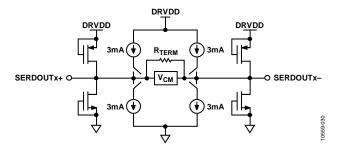
Figure 30. Digital CML Output Circuit
