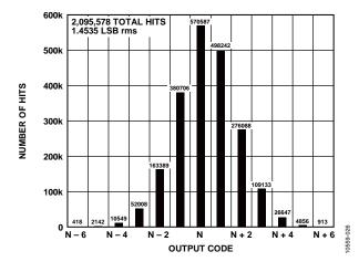
Figure 26. AD9250-250 Grounded Input Histogram
