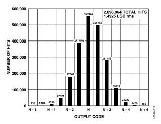
Figure 15. AD9250-170 Grounded Input Histogram
