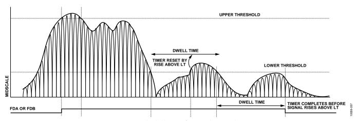
Figure 61. Threshold Settings for FDA and FDB Signals
