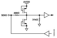
Figure 31. Equivalent SDIO Circuit
