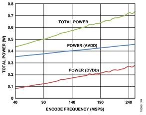
Figure 53. AD9250-250 Power vs. Encode Rate
