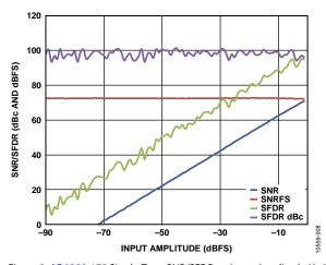
Figure 8. AD9250-170 Single-Tone SNR/SFDR vs. Input Amplitude ( $A_{\rm IN}$ ) with  $f_{\rm IN}$  = 185.1 MHz
