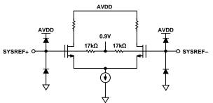
Figure 34. Equivalent SYSREF± Input Circuit
