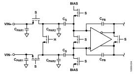
Figure 38. Switched-Capacitor Input
