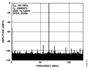
Figure 17. AD9250-250 Single-Tone FFT with  $f_{IN} = 185.1$  MHz
