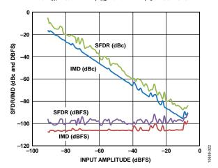
Figure 22. AD9250-250 Two-Tone SFDR/IMD vs. Input Amplitude ( $A_{IN}$ ) with  $f_{INI} = 184.12$  MHz,  $f_{IN2} = 187.12$  MHz,  $f_S = 250$  MSPS
