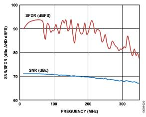
Figure 20. AD9250-250 Single-Tone SNR/SFDR vs. Input Frequency (f<sub>IN</sub>)
