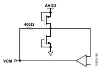
Figure 36. Equivalent VCM Circuit
