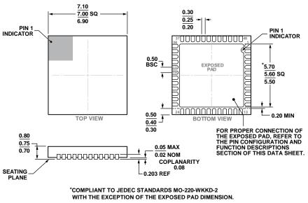
Figure 63. 48-Lead Lead Frame Chip Scale Package [LFCSP\_WQ] 7 mm × 7 mm Body, Very Very Thin Quad (CP-48-13) Dimensions shown in millimeters
