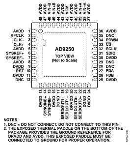
Figure 4. Pin Configuration (Top View)
