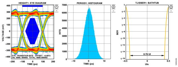
Figure 59. AD9250 Digital Outputs Data Eye, Histogram and Bathtub, External 100  $\Omega$  Terminations at 5 Gbps
