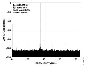
Figure 7. AD9250-170 Single-Tone FFT with  $f_{IN} = 305.1$  MHz
