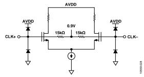
Figure 28. Equivalent Clock Input Circuit
