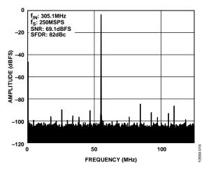
Figure 18. AD9250-250 Single-Tone FFT with  $f_{IN}$  = 305.1 MHz
