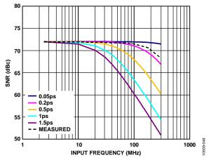
Figure 52. AD9250-250 SNR vs. Input Frequency and Jitter
