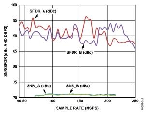
Figure 25. AD9250-250 Single-Tone SNR/SFDR vs. Sample Rate ( $f_s$ ) with  $f_{\rm IN}$  = 90.1 MHz
