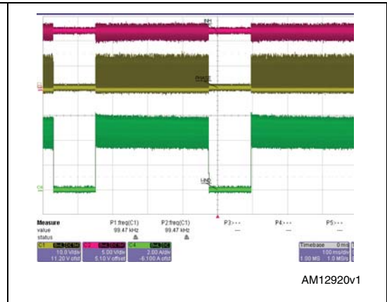
Figure 31. Thermal shutdown protection
