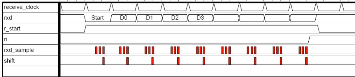
Fig. 7-4: Receive mode 1 for Serial 0
