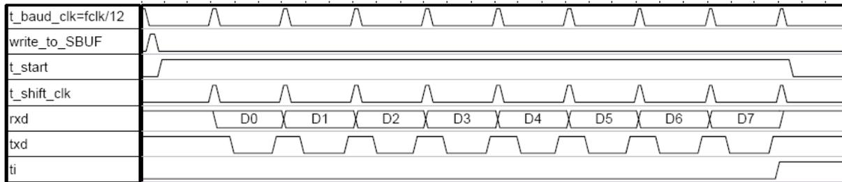
Fig. 7-1: Transmit mode 0 for Serial 0
