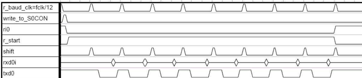
Fig. 7-2: Receive mode 0 for Serial 0
