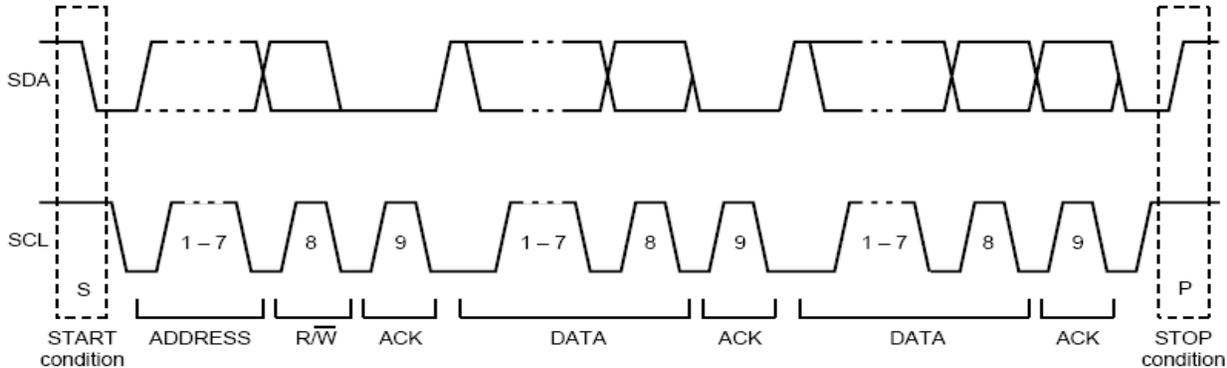
Fig. 11-2: RW bit in the 8<sup>th</sup> bit after IIC address
