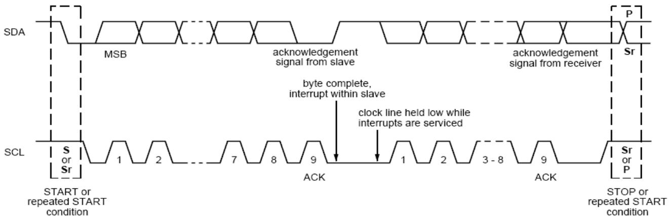
Fig. 11-1: Acknowledgement bit in the 9<sup>th</sup> bit of a byte transmission
