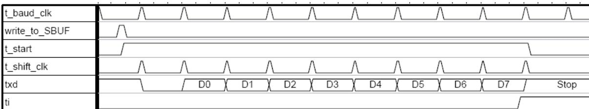
Fig. 7-3: Transmit mode 1 for Serial 0
