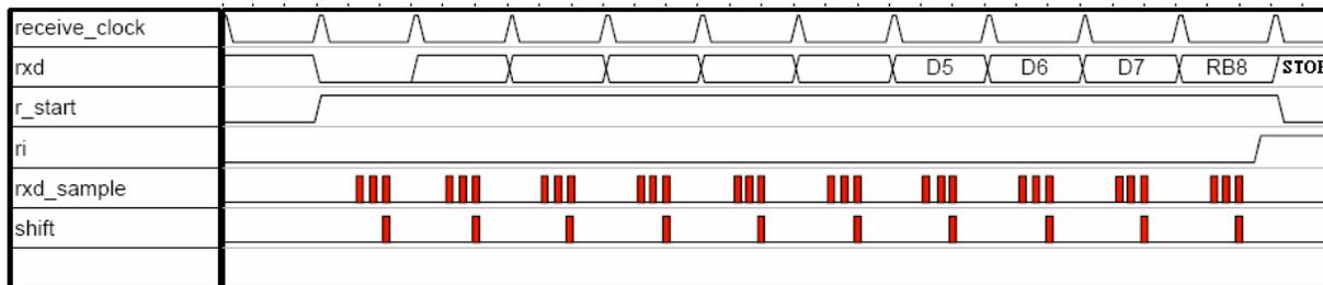
Fig. 7-6: Receive modes 2 and 3 for Serial 0
