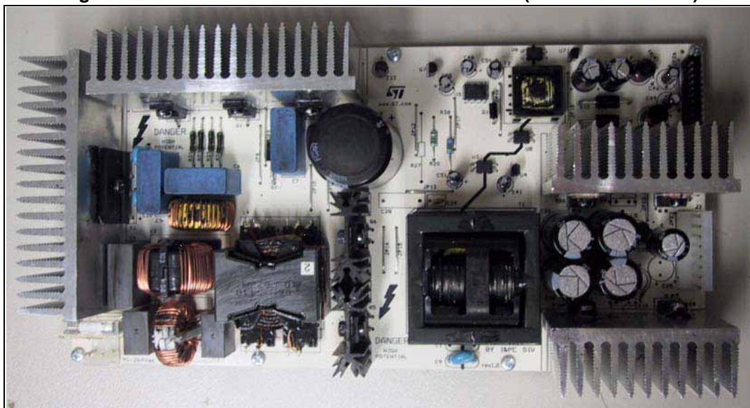
Figure 19. L6599 and L6563 400 W evaluation board (EVAL6599-400W-S)
