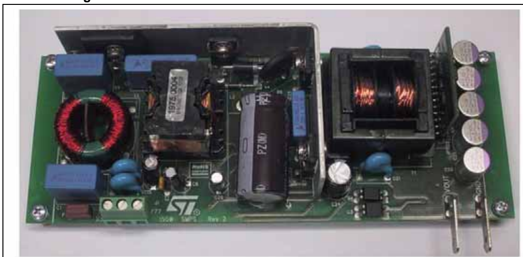
Figure 9. EVL6699-150W-SR 150 W SMPS demonstration board
