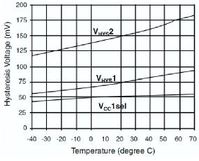
Figure 5. Hysteresis Voltage vs. Temperature
