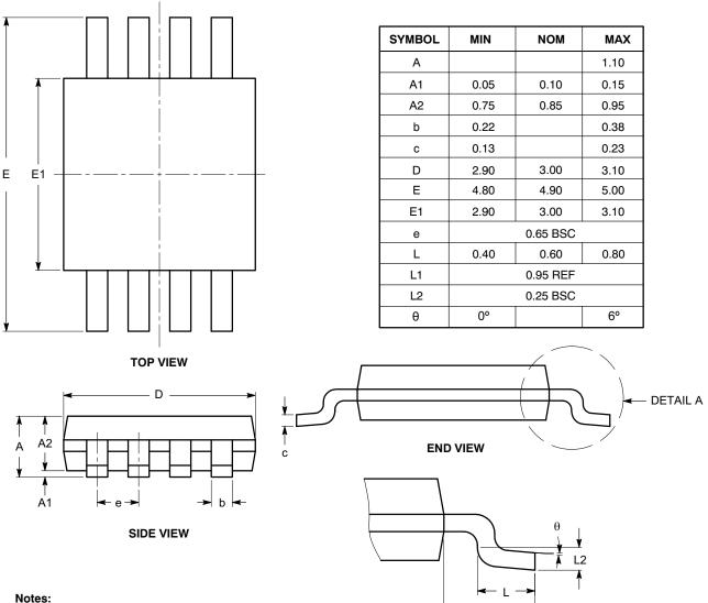
(1) All dimensions are in millimeters. Angles in degrees.
