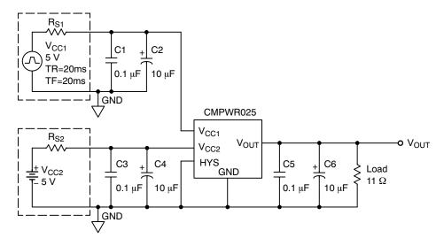
Figure 6. Transient Characterization Test Set-Up
