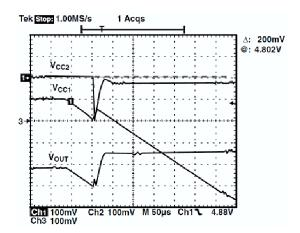
Figure 8.  $V_{CC1}$  Falling form 0 V to 5 V ( $V_{CC2}$  = 5 V). Ch1 and Ch2: V<sub>CC1</sub> and V<sub>CC2</sub>, offset = 5 V. Ch3: V<sub>OUT</sub>, offset = 5 V.
