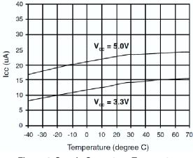
Figure 4. Supply Current vs. Temperature
