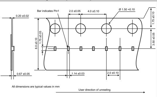
Figure 13. Tape and reel specifications
