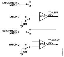
Figure 33. Single-Ended Input Configuration
