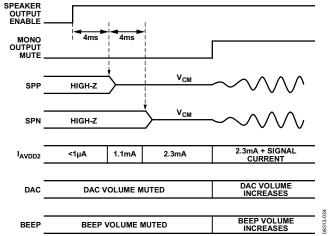
Figure 36. Speaker Driver Power-Up Sequence
