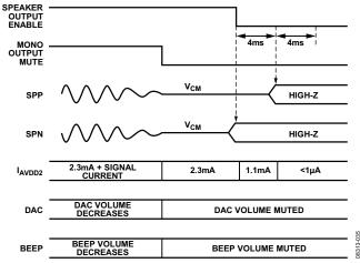
Figure 37. Speaker Driver Power-Down Sequence
