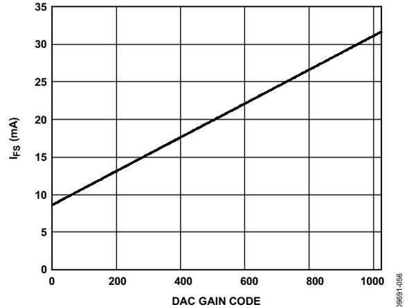
Figure 51. DAC Full-Scale Current vs. DAC Gain Code
