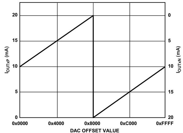
Figure 45. DAC Output Currents vs. DAC Offset Value
