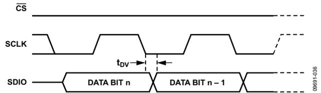
Figure 29. Timing Diagram for Serial Port Register Read
