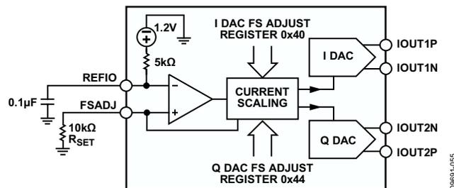
Figure 50. Simplified Block Diagram of DAC Core
