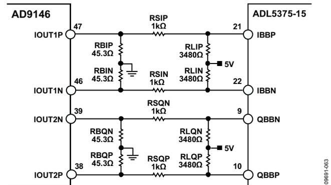
Figure 57. Passive, Level-Shifting Network for Biasing the ADL5375-15
