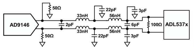
Figure 58. DAC Modulator Interface with Fifth-Order, Low-Pass Filter
