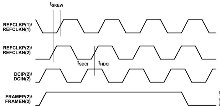
Figure 63. Timing Diagram Required for Synchronizing Devices
