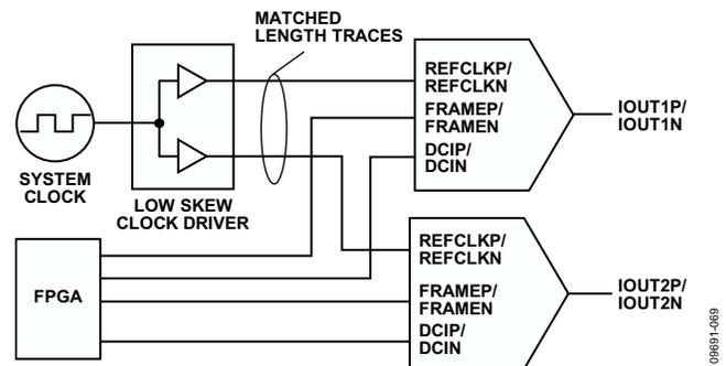
Figure 62. Typical Circuit Diagram for Synchronizing Devices
