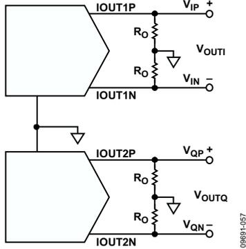
Figure 52. Basic Transmit DAC Output Circuit
