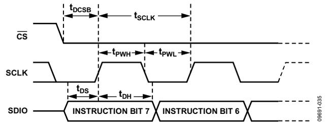
Figure 28. Timing Diagram for Serial Port Register Write
