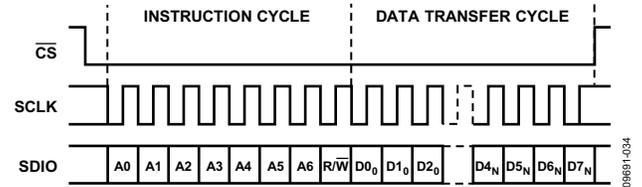
Figure 27. Serial Port Interface Timing, LSB First
