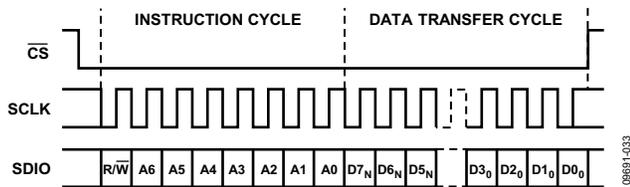
Figure 26. Serial Port Interface Timing, MSB First
