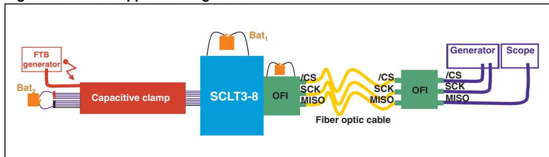
Figure 40 shows the output MISO behavior is not disturbed during fast transient bursts. The FTB signal has been captured through an antenna to observe where the bursts act.
