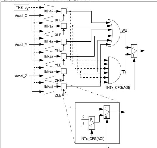
Figure 8. Free-fall, wake-up interrupt generator
