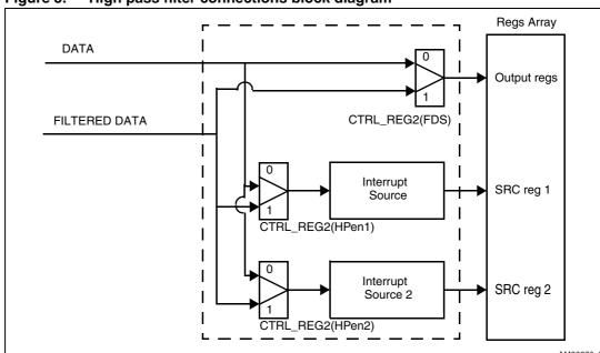
Figure 5. High pass filter connections block diagram
