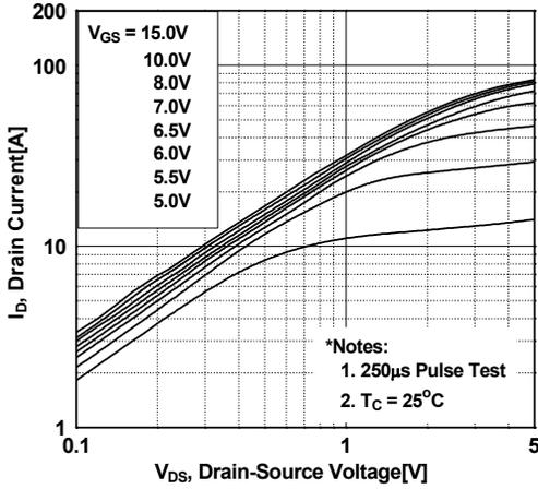
**Figure 2. Transfer Characteristics**
