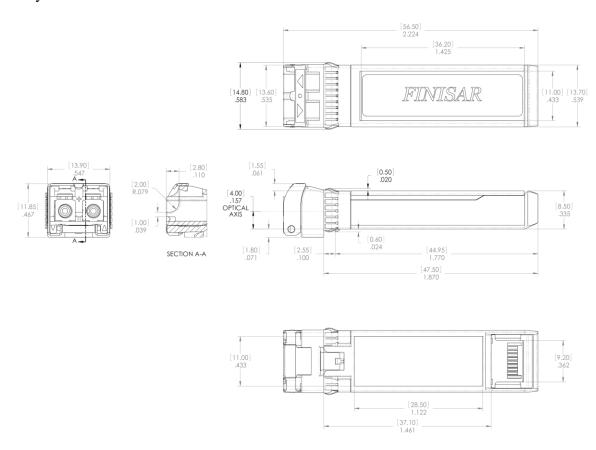
Figure 2. FTLX8573D3BTL Mechanical Dimensions.
