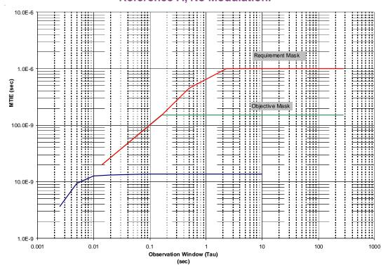
\*NOTE: The wider bandwidth of this model may result in a break in the GR-253-CORE, R5-135 Switching Mask for observation times of <50ms.
