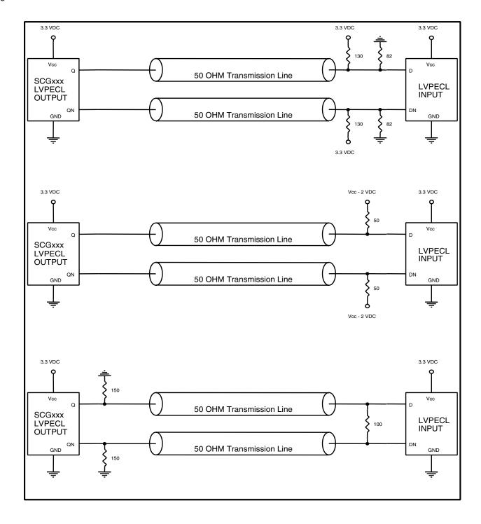
If PECL outputs do not drive a long line (< 0.5"), a single  $150\Omega$  termination resistor to ground may be used for each pin.
