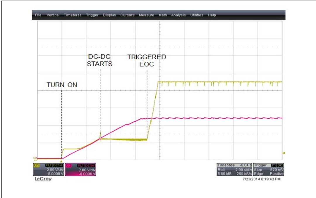
Figure 13. Buck-boost startup ( I_{IN} = 5\ \mu\text{A} )
