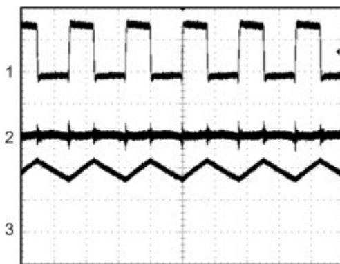
Heavy Load Mode Output Voltage Ripple
