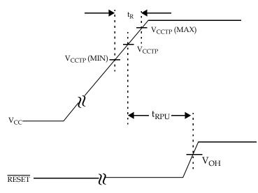
Figure 1: Timing Diagram: Power-Up
