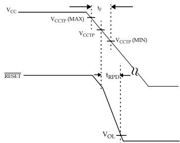
Figure 2: Timing Diagram: Power-Down
