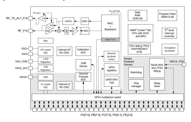
Figure 4.1. EM359x Block Diagram
