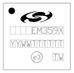
Figure 6.4. Part Marking for EM359x
