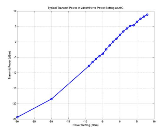
Figure 3.2. Transmit Output Power
