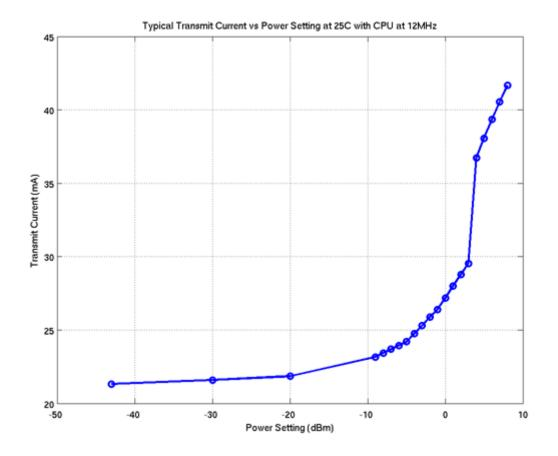
**Figure 3.1. Transmit Power Consumption**
