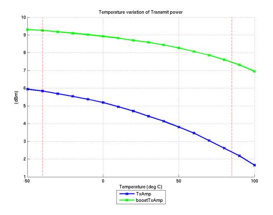
Figure 3.4. Transmit Power vs. Temperature
