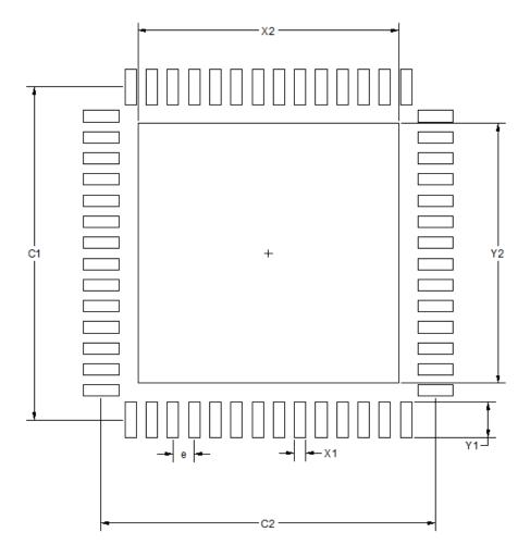
Figure 6.3. Solder Mask Dimensions
