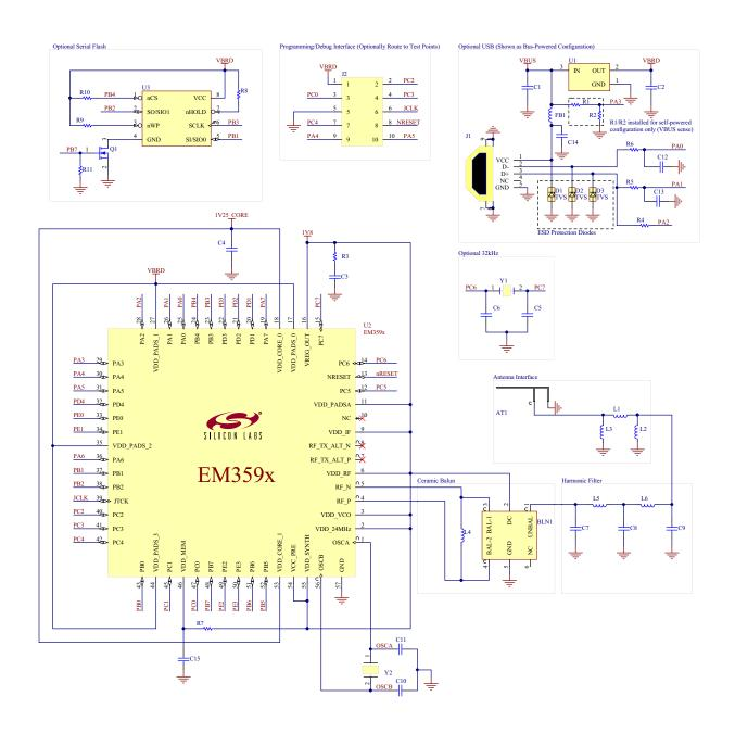
Figure 2.1. Typical Application Circuit
