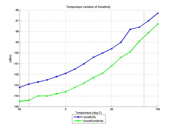
Figure 3.3. Receive Sensitivity vs. Temperature
