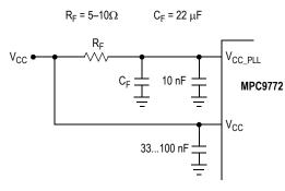
Figure 7. V<sub>CC PLL</sub> Power Supply Filter
