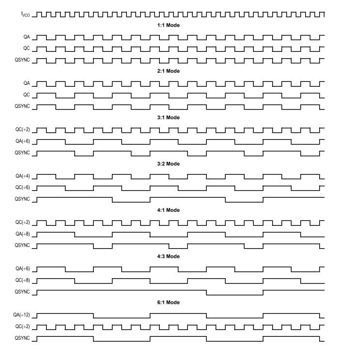
Figure 6. QSYNC Timing Diagram
