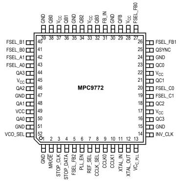
Figure 2. MPC9772 52-Lead Package Pinout (Top View)
