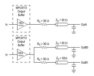
Figure 12. Single versus Dual Transmission Lines
