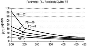
Max. I/O Phase Jitter versus Frequency
