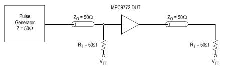
Figure 15. CCLK MPC9772 AC Test Reference
