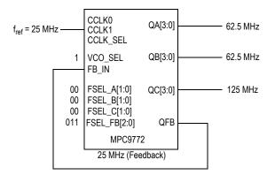
MPC9772 example configuration (feedback of QFB = 25 MHz,  $f_{VCO}$ =250 MHz, VCO\_SEL=÷1, M=10, N<sub>A</sub>=4, N<sub>B</sub>=4, N<sub>C</sub>=2).
