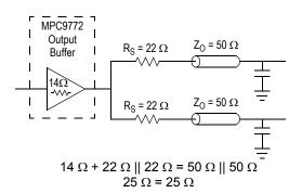
Figure 14. Optimized Dual Line Termination
