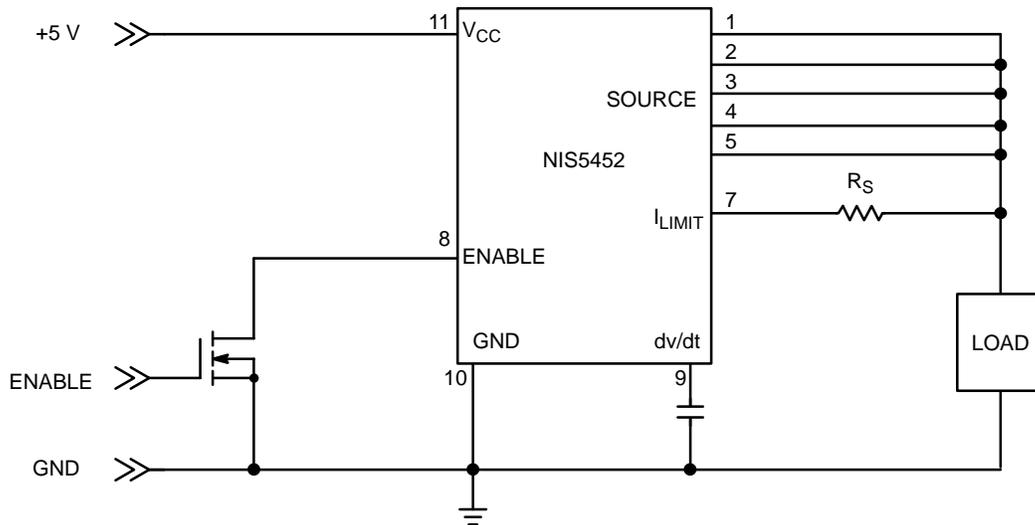
Figure 2. Application Circuit with Direct Current Sensing
