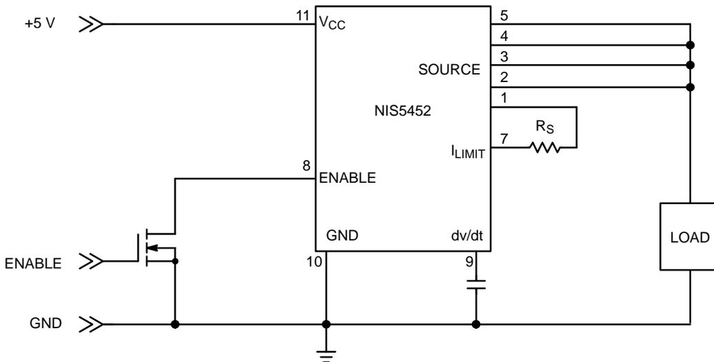
Figure 3. Application Circuit with Kelvin Current Sensing
