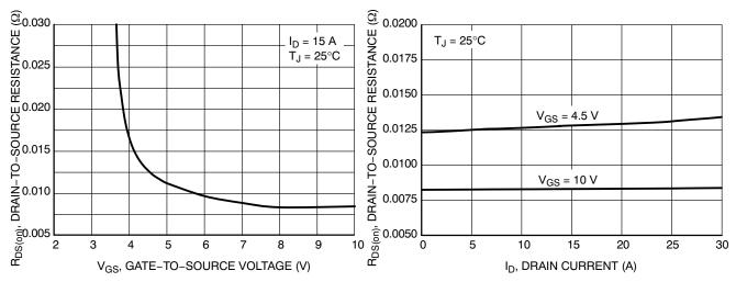
Figure 3. On-Resistance vs. V<sub>GS</sub>
