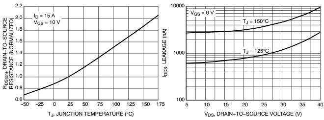
Figure 5. On–Resistance Variation with Temperature
