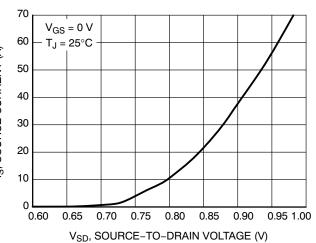
Figure 10. Diode Forward Voltage vs. Current
