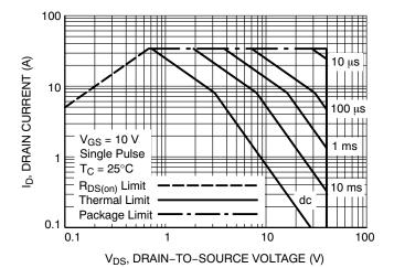
Figure 11. Maximum Rated Forward Biased Safe Operating Area
