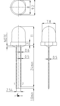
Units: mm / tolerance = +/-0.1mm
