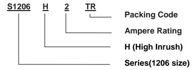
Note: TR: 3,000 pieces of fuses on 8mm tape-and-reel on a 7 inch (178mm) reel per EIA Standard 481
