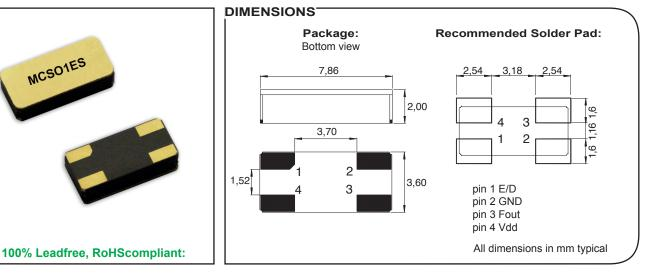
SC cut quartz crystal SMT Clock oscillator in ceramic package Fundamental quartz mode frequency Ultra low stability High shock and vibration resistance Wide temperature range Low aging Ultra low MSL Very fast start-up Excellent solderability Swiss made quality Customer specification on request
