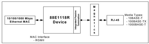
88E1118R Device used in Copper Application
