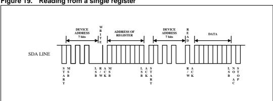
Figure 19. Reading from a single register
