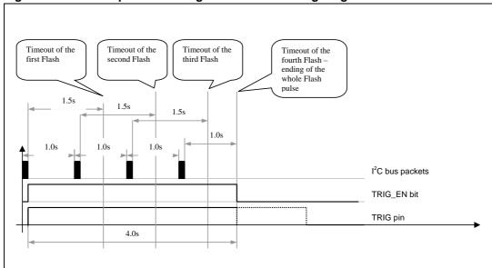
Figure 22. I<sup>2</sup>C bus packets timing for a FLASH lasting longer than FTIM max
