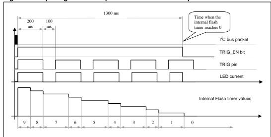
Figure 16. Splitting the FLASH pulse into several shorter pulses
