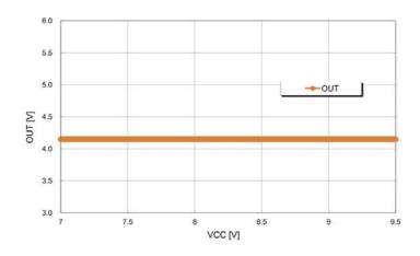
Figure 15. OUT(27,28,35~40pin)\_DC-Bias = 4.15V fixed.
