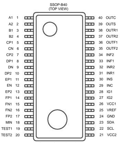
Figure 2. Pin configuration
