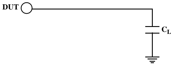
Figure 10. Output Test Load Circuit for LOCK and Dynamic Power Supply Current Measurements
