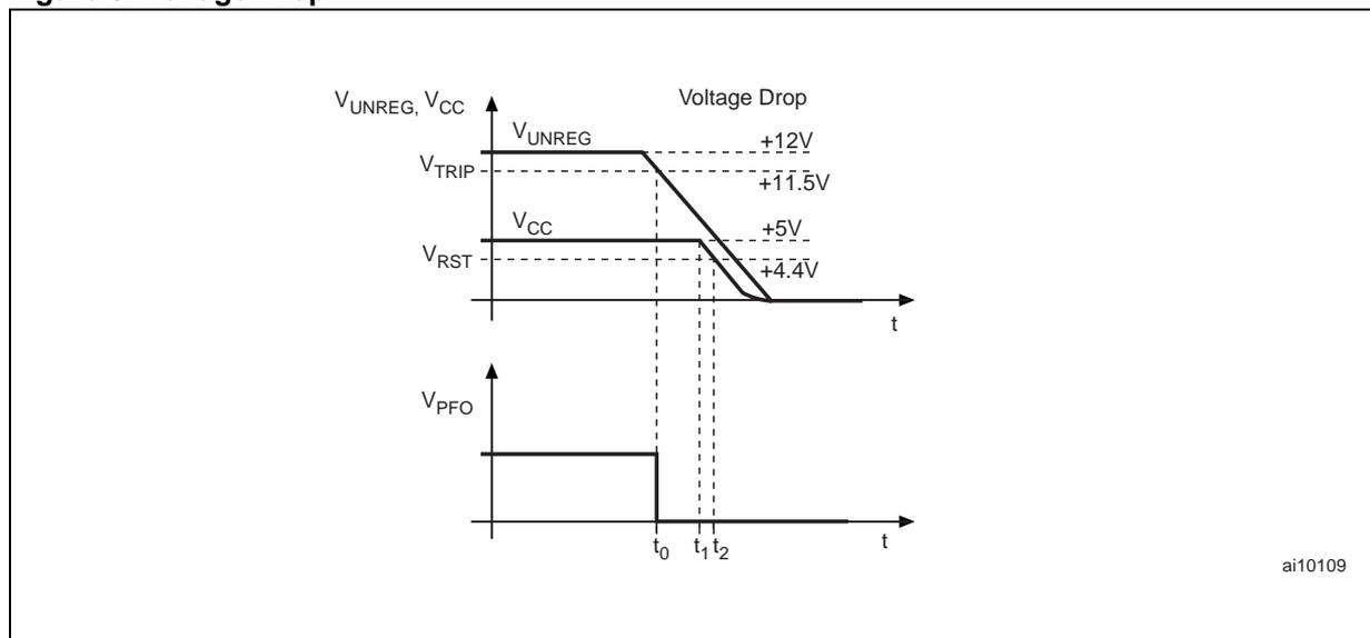
Note: At  $t_0$  the voltage drop is detected; at  $t_1$   $V_{CC}$  begins to fall; at  $t_2$  Reset is asserted and/or Write Protect occurs.
