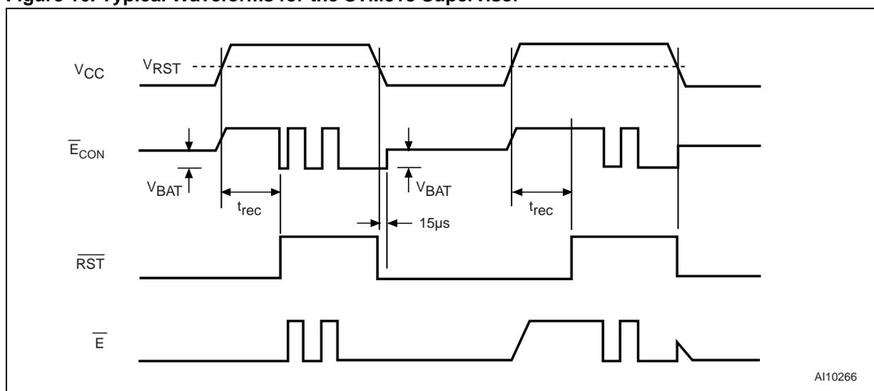
Note: The chip enable gating function is also implemented on the STM795 device. Nevertheless there are two differences, in comparison to the STM818. Firstly the  $\overline{E}_{CON}$  signal is held High only for half of the  $t_{REC}$  period, and secondly the chip-enable transmission gate is disabled only 10 $\mu$ s after Reset is asserted if the  $\overline{E}$  input is Low.
