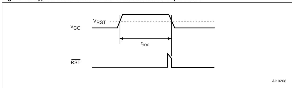
Note: 1. For the STM818,  $\overline{ECON}$  is held Low, externally. The  $\overline{ECON}$  state is latched half way through the  $t_{REC}$  period, and the Freshness Seal function is enabled.
