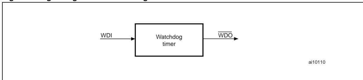
Note: 1. WDI is the Watchdog Input,  $\overline{\text{WDO}}$  is the Watchdog Output.
