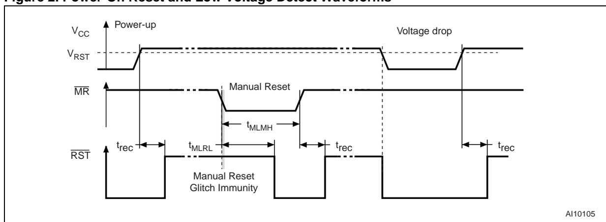
Note:  $V_{RST}$  is the Reset threshold, see [Table 3](#). for values.
