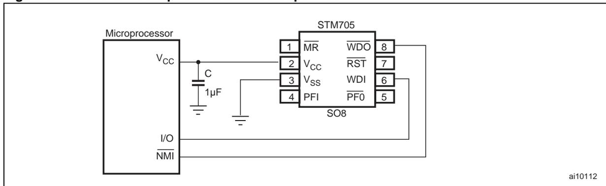
In any case, if V<sub>CC</sub> drops below the Reset threshold (V<sub>RST</sub>),  $\overline{WDO}$  goes Low even if the watchdog timer has not timed out. The timer remains cleared and does not count for as long as Reset is asserted. The counter automatically restarts after t<sub>rec</sub> expires.
