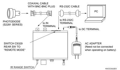
Note: Use the Rf RANGE switch to change the detection sensitivity. (Detection sensitivity cannot be changed from the PC.)
