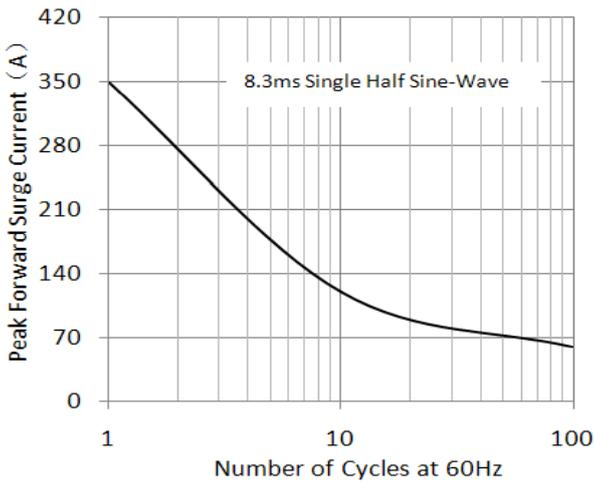
Figure 3. Maximum Non-Repetitive Peak Forward Surge Current
