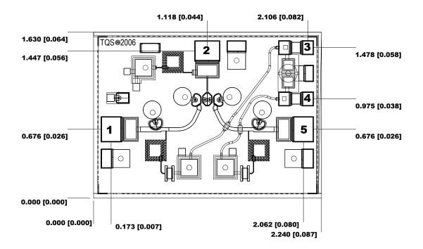
Units: millimeters (inches) Thickness: 0.100 (0.004) Chip edge to bond pad dimensions are shown to center of bond pad Chip size tolerance: +/- 0.051 (0.002)
