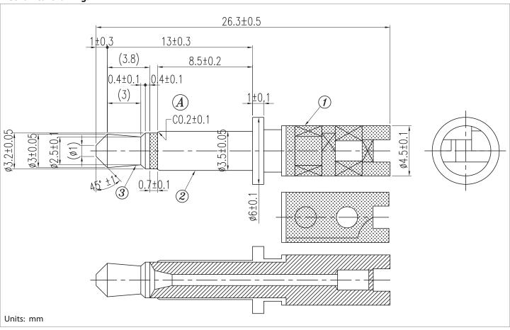
tolerance X:  $\pm 0.5 \, \text{mm}$  .X:  $\pm 0.3 \, \text{mm}$  .XX:  $\pm 0.05 \, \text{mm}$  applicable unless otherwise indicated in specification or on drawings
