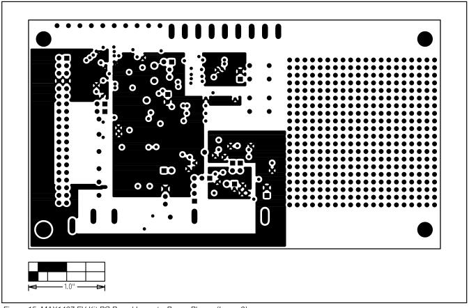
Figure 15. MAX1407 EV Kit PC Board Layout—Power Planes (Layer 3)
