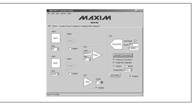
Figure 2. ADC Control Panel
