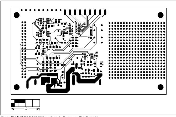
Figure 13. MAX1407 EV Kit PC Board Layout—Component Side (Layer 1)
