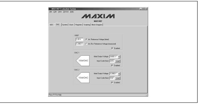
Figure 3. DAC Control Panel
