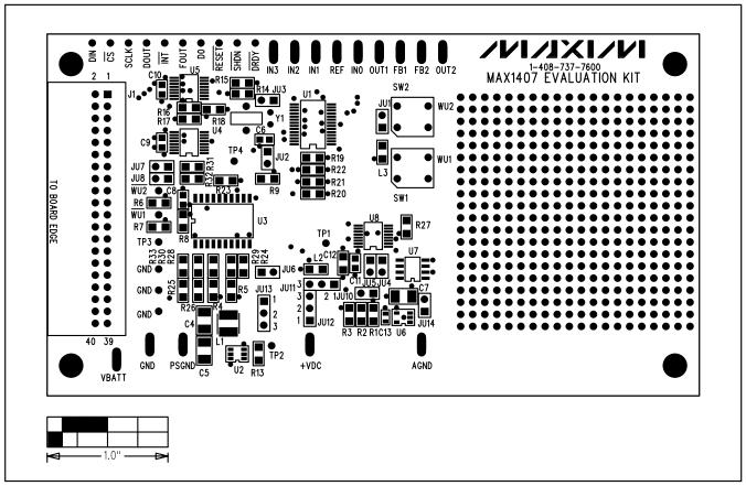
Figure 11. MAX1407 EV Kit Component Placement Guide—Component Side
