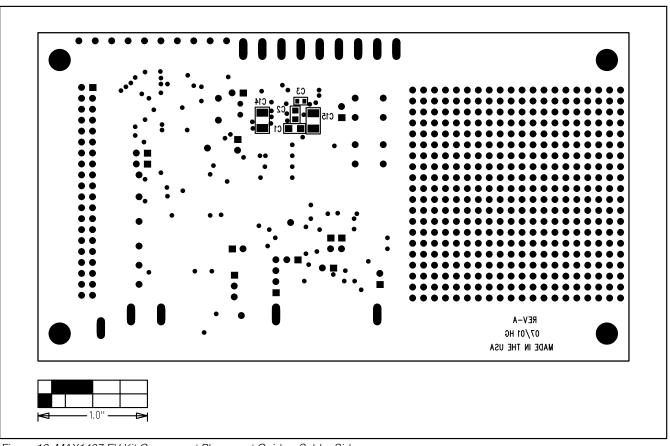
Figure 12. MAX1407 EV Kit Component Placement Guide—Solder Side
