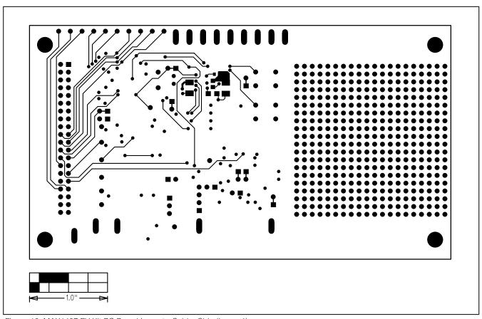
Figure 16. MAX1407 EV Kit PC Board Layout—Solder Side (Layer 4)
