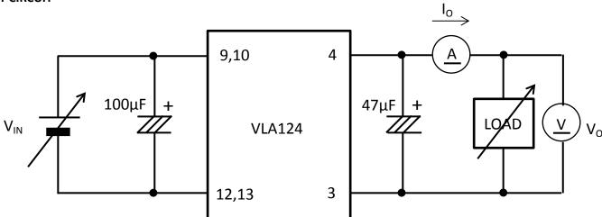
★It is used the electrolytic capacitors which has the low impedance for output capacitor.
