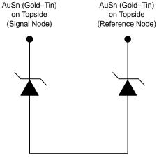
Silicon Substrate on Backside
