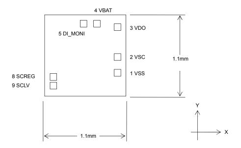
Chip size :  $1.1 \text{mm} \times 1.1 \text{mm}$ The number of pads : 7 pinsMinimum pad pitch :  $120 \text{ } \mu\text{m}$ Pad opening :  $90 \text{ } \mu\text{m} \times 90 \text{ } \mu\text{m}$ Chip thickness :  $350 \text{ } \mu\text{m}$
