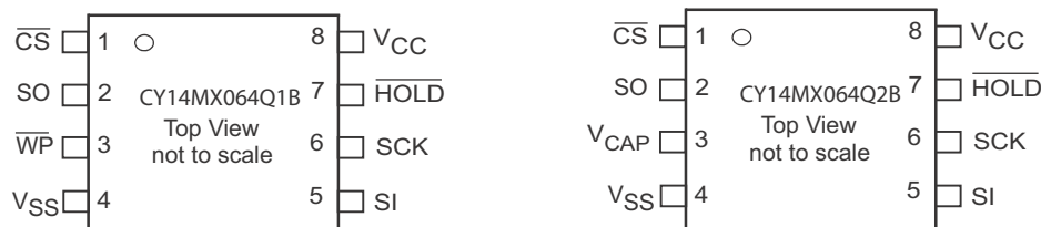
Figure 1. 8-pin SOIC pinout [1, 2]
