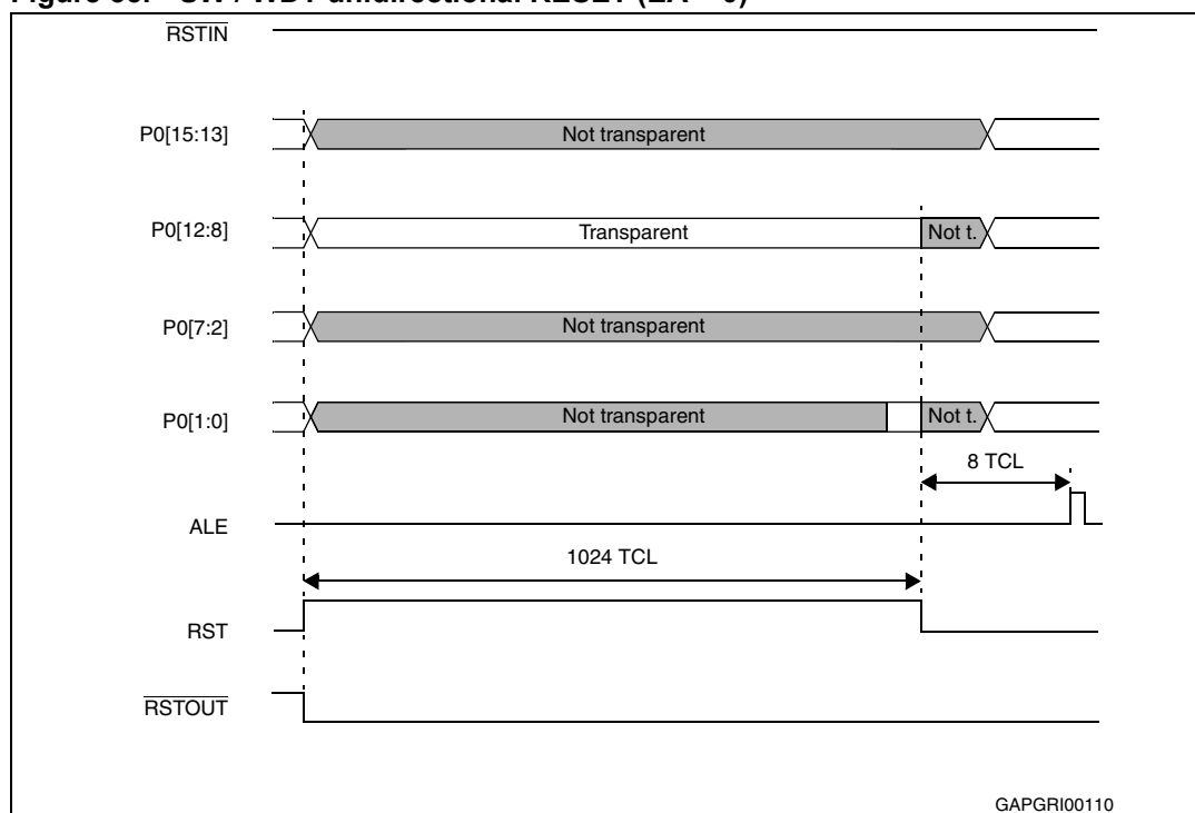
Figure 33. SW / WDT unidirectional RESET ( \overline{EA} = 0 )
