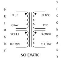
Primary and secondary windings are designed to be connected in series or parallel. Windings are not intended to be used independently.
