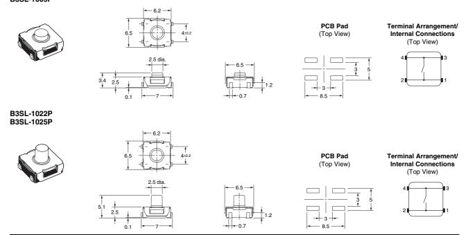
Note: Unless otherwise specified, a tolerance of ±0.4 mm applies to all dimensions. No terminal numbers are indicated on the Switches.
