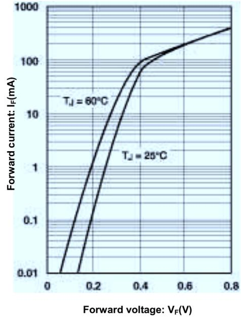
Figure 2. Forward characteristics
