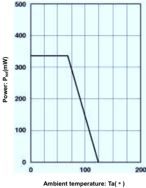
Figure 1. Admissible power dissipation vs. ambient temperature
