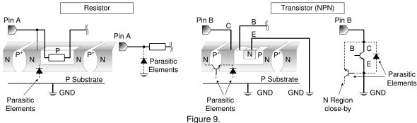
Example of monolithic IC structure
