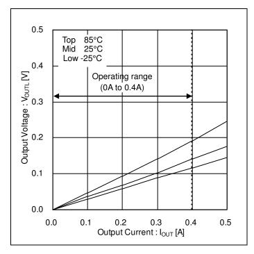
Figure 3. Low Side Output Voltage vs Output Current
