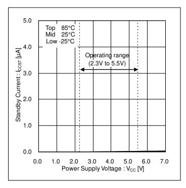
Figure 1. Standby Current vs Supply Voltage
