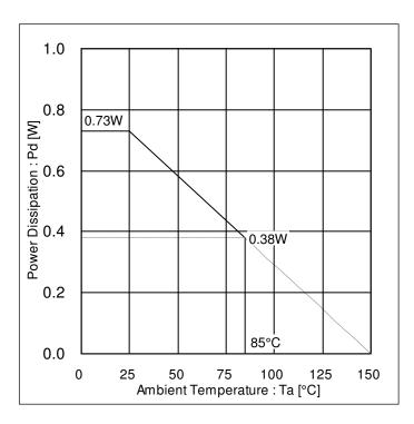
Figure 8. Power Dissipation vs Ambient Temperature
