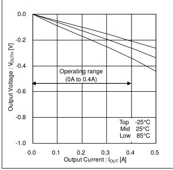
Figure 4. High Side Output Voltage vs Output Current
