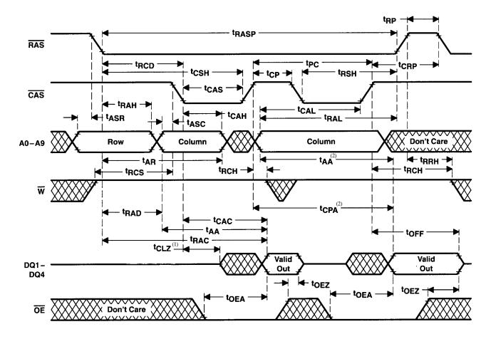
L. Valid data is presented at the outputs after all access times are satisfied but can go from the high-impedance state to an invalid-data state prior to the specified access tiems as the outputs are driven when CAS\ and OE\ are low.
